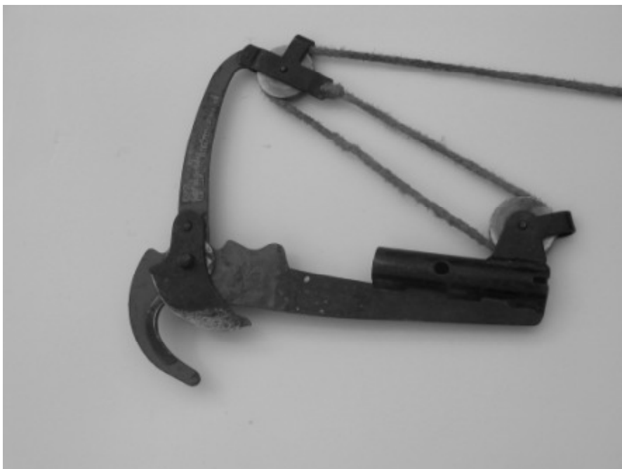
Image 2. A pruner by Sandvik with pulleys operated by ropes.
